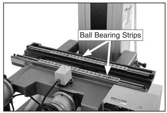
Figure 16. Ball bearing strips positioned on saddle ways.
